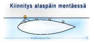
Mooring when going downstream: Tie the loop from the aft of the boat. If no other boats are in the lock, use the first available floating bollard for mooring.
