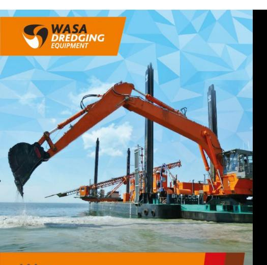
Wasa BOULDER Backhoe Dredger / Drill Pontoon
