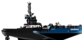
Calypso Saimaa combination 2020 L. 40.8m B. 12.6m Power 2 600kW
