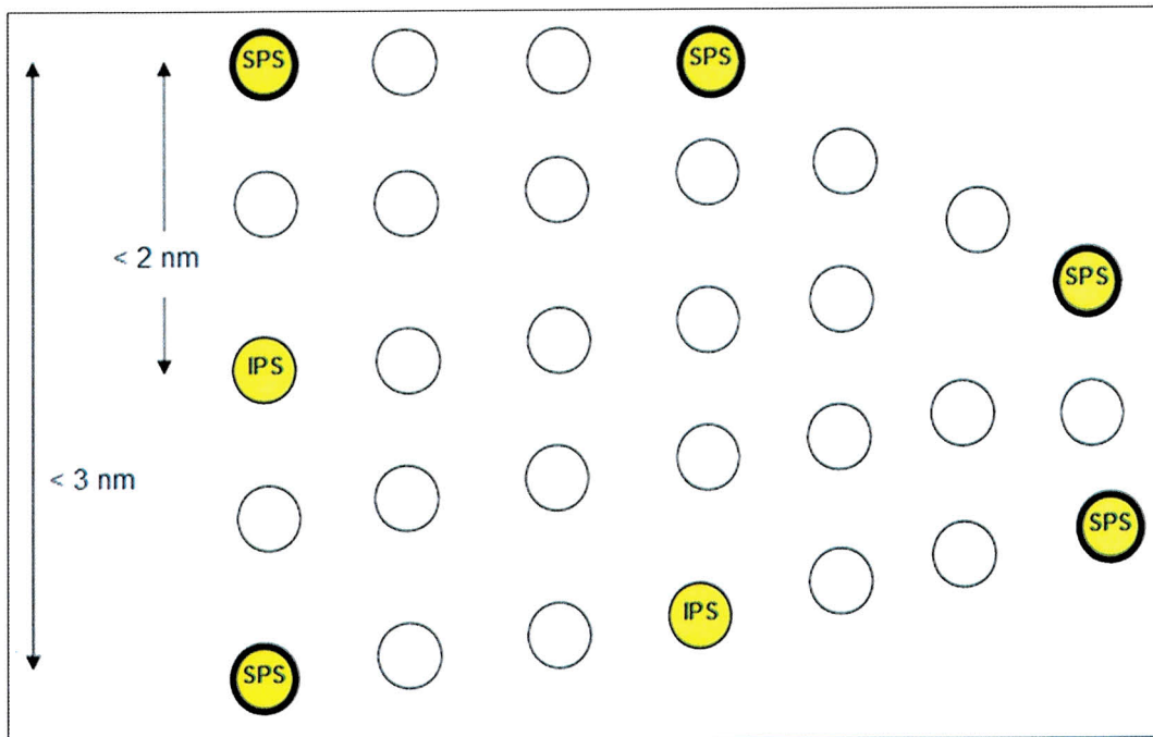
Picture 6 Example of marking a wind farm (IALA recommendation, The marking of offshore man-made structures, 2021). In addition, individual wind turbines (IPS) can be marked between the corner wind turbines (SPS); their light markings must differ clearly from the light markings of the corner wind turbines.
