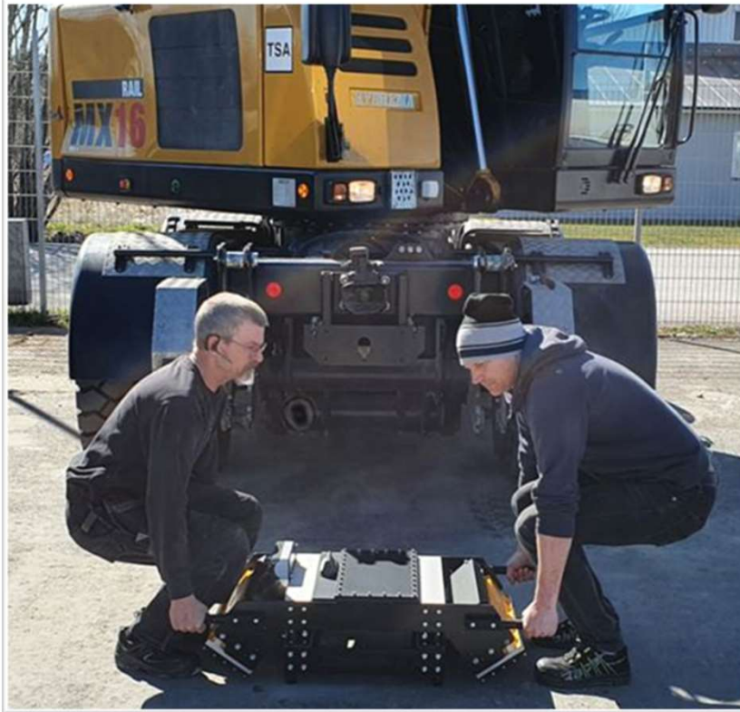
Step 1, Lift LTM to pre-assembled bracket
