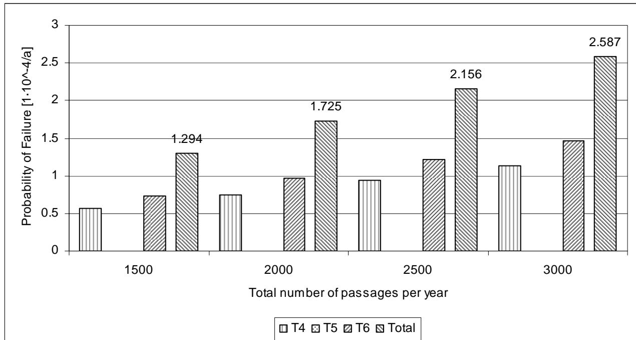
*Figure 5 Probability of failure for different vessel speeds (foundation capacities see Table 2, ship speed 9 knots).*
