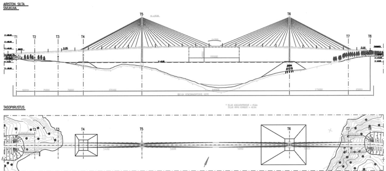
*Figure 8 Airisto Cable Stayed Bridge including protection islands for pier T4 and pylon T5*
