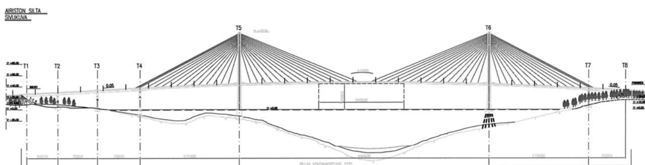
*Figure 1 Elevation of general bridge arrangement.*
