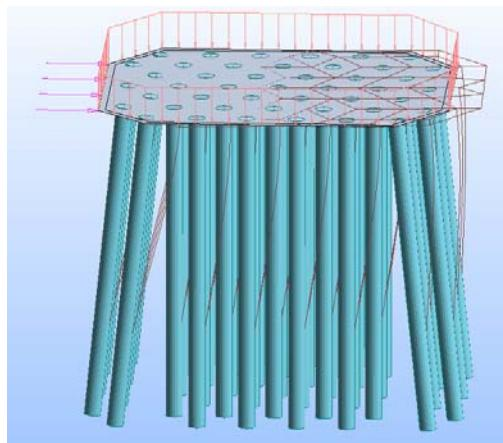
Figure 3 Arrangement of pile foundation for pylon T6
