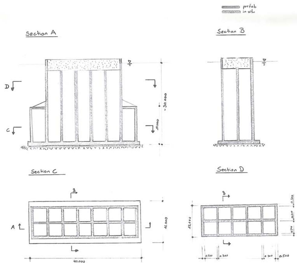
Figure 11 Caisson solution for the foundation of pylon T6.
