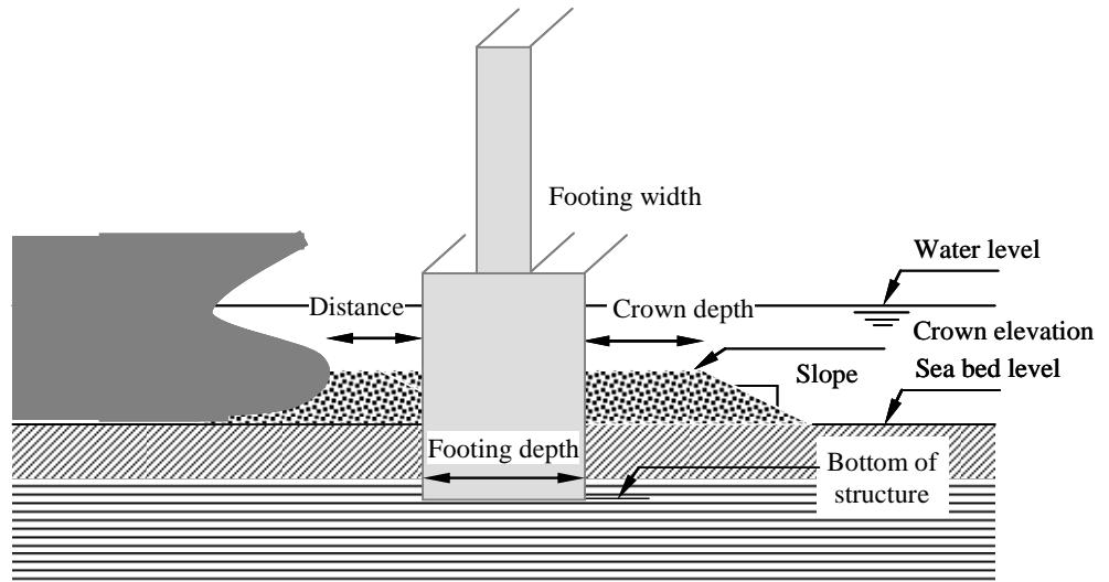
Figure 7 Geometrical overview of ship grounding on protection islands.
