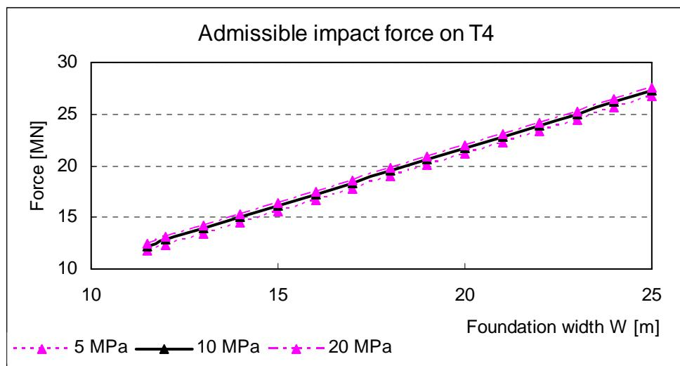
Figure 9 Increase of horizontal capacity for slab foundation of pier T4.
