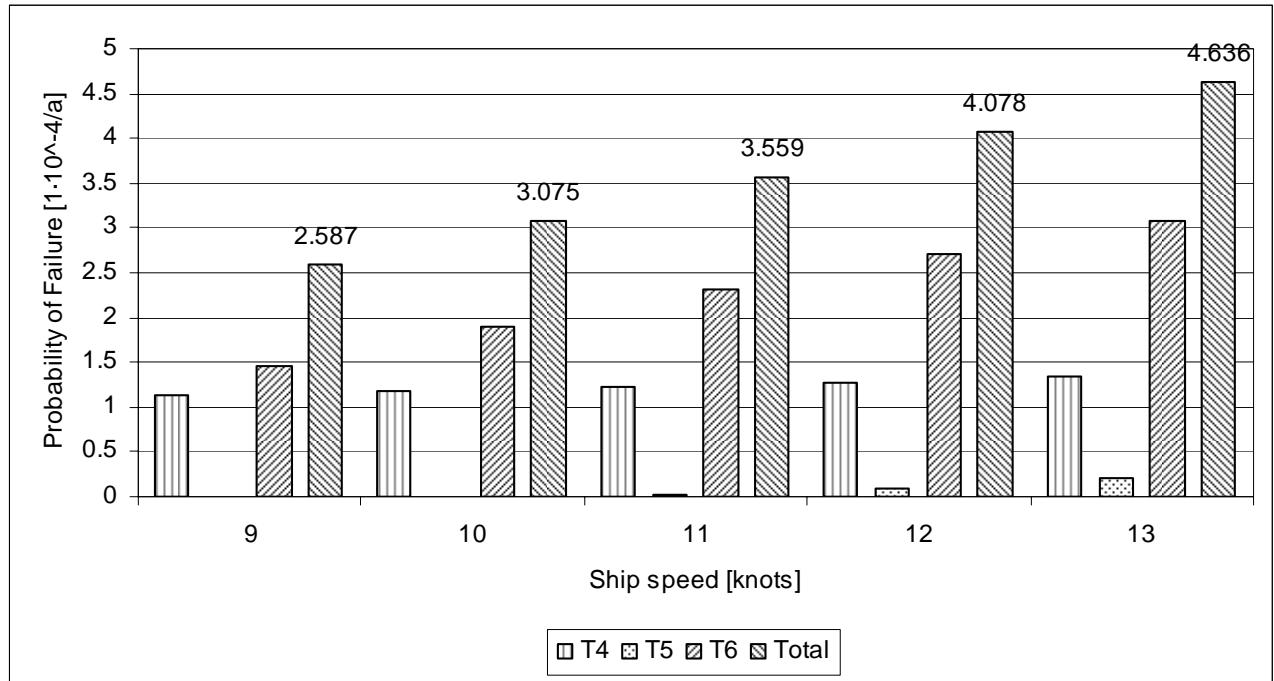
*Figure 4 Probability of failure for different vessel speeds (foundation capacities see Table 2, 3000 ships/year).*
