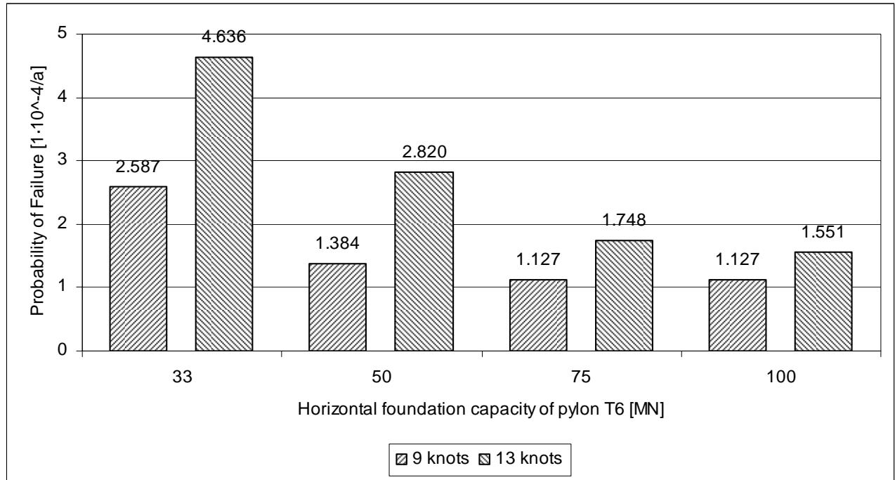
*Figure 6 Influence of the horizontal foundation capacity of pylon T6 on the total risk of ship impact*
