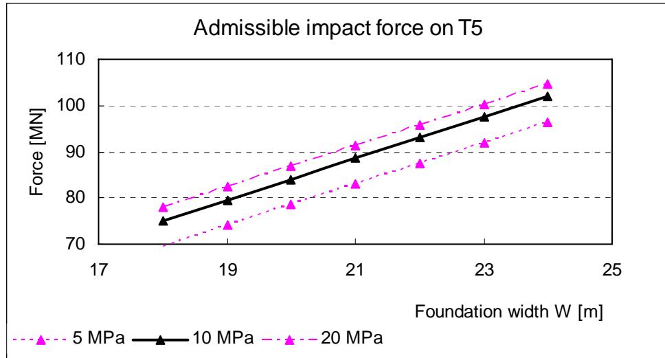
Figure 10 Increase of horizontal capacity for slab foundation of pylon T5.
